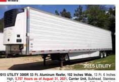
2015 UTILITY 3000R 53 Ft. Aluminum Reefer, 102 Inches Wide, 13 Ft. 6 Inches High, 5,767 Hours as of August 31, 2021, Carrier Unit, Bulkhead, Stainless Steel Front Corners, White Lined, Cold Chute, Aluminum Scuff Plate, Rear Vent, Stainless Steel Door Frame & Buck Plate, Stainless Steel Swing Doors, Under Trailer Wind Deffector, Stainless Steel ICC Bumper, Dock Locks, Air Release Sliding Tandem, Air Ride Suspension, PSI Tire Inflation System, 22.5 Low Profile Tires, Aluminum Disc Wheels
