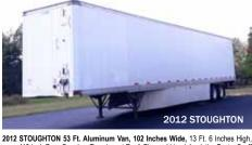
110 Inch Door Opening, Translucent Roof, Plywood Lined, Logistics Posts, Scuff Board, Threshold Plate, Front & Rear Vents, Galvanized Door Frame & Buck Plate, Swing Doors, Under Trailer Wind Deflector, Dock Locks, Galvanized ICC
