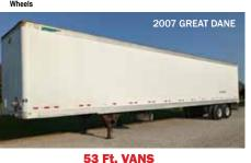
2007 GREAT DANE 53 Ft. Aluminum Van, 102 Inches Wide, 13 Ft. 6 Inches High, 110 Inch Door Opening, Translucent Roof, Plywood Lined, Logistics Posts, Scuff Plate, Threshold Plate, Swing Doors, Sliding Tandem, Air Ride Suspension, 22.5 Low Profile Tires, Disc Wheels
