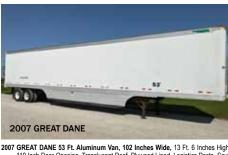
2007 GREAT DANE 53 Ft. Aluminum Van, 102 Inches Wide, 13 Ft. 6 Inches High, 110 Inch Door Opening, Translucent Roof, Plywood Lined, Logistics Posts, Scuff Plate, Threshold Plate, Swing Doors, **Under Trailer Wind Deflector**, Sliding Tandem, **Air Ride Suspension**, 22.5 Low Profile Tires, Disc Wheels
