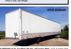
2005 WABASH 53 Ft. DuraPlate HD Van, 102 Inches Wide, 13 Ft. 6 Inches High, 110 Inch Door Opening, Translucent Roof, Logistics Equipped, Aluminum Scuff Plate, Threshold Plate, Stainless Steel Door Frame & Buck Plate, Swing Doors, Stainless Steel Co Bumper, Stilling Tandem, Air Ride Suspension, Tire Inflation System, 22.5 Low Profile Tires, Disc Wheels
